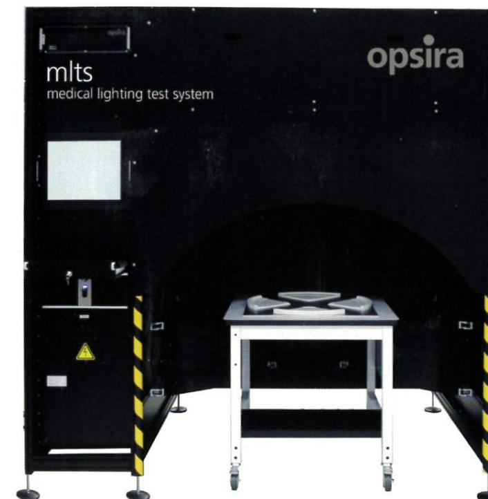
The test system for medical lighting mlts is based on the system add-on luca'lux for fast measurements with high resolution and test of illuminance distributions by a photometrically corrected measuring camera. The photometric and geometric measurement of the light field is done within seconds and tested against the respective standards (e.g. DIN EN 60601-2-41).
