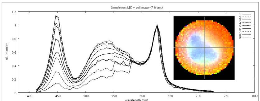
**Figure 9:** Simulated spectra of LED package and collimator based on raydata generated with 7 bandpass filters. Inset: Simulated light distribution on the screen
