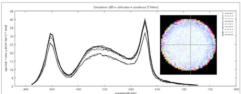
**Figure 11:** Simulated spectra of LED package, collimator, and condenser based on raydata generated with 7 bandpass filters. Inset: Simulated light distribution on the screen
