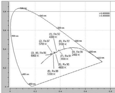
coordinates being close to the Planck curve. CRIs  $R_a$  vary between 92 and 86 with the one from the  $V(\lambda)$  simulation reaching a value of 89. These values can then be used in further application design if necessary.
