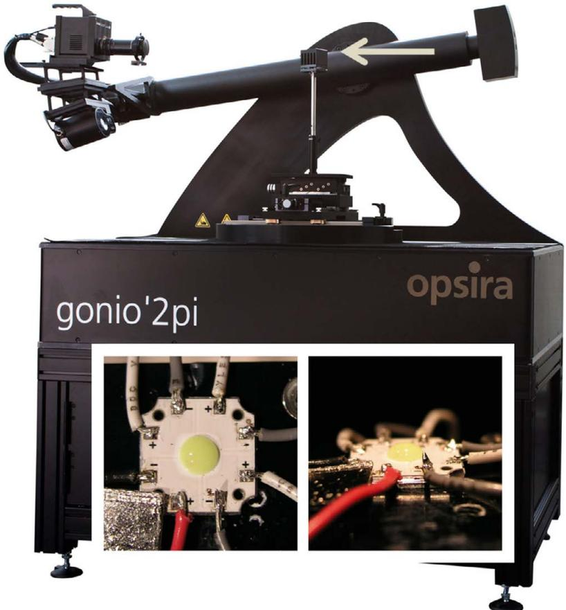
varies for different observation angles. Also, the spectrum depends on the point of origin on the light source and varies with the proximity to, e.g., a blue or red chip. These characteristics need to be accounted for in the data.
