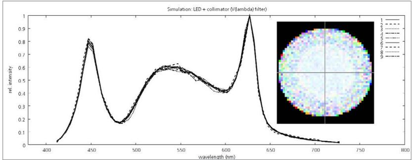
the red diode. The spectra are normalized to the height of the red peak to show how the blue / red ratio decreases as we go from the blue to the red region on the screen.
